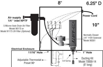
Electrical conduit can be attached to the system box but requires a suitable connector rather than the grip tight connector
