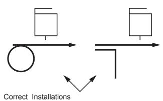
\*NOTE: In some cases only a small amount of open air is needed for effective static neutralization over a grounded object. Examples: Over a stack of sheets while feeding, or on a feedboard of a printing press.
